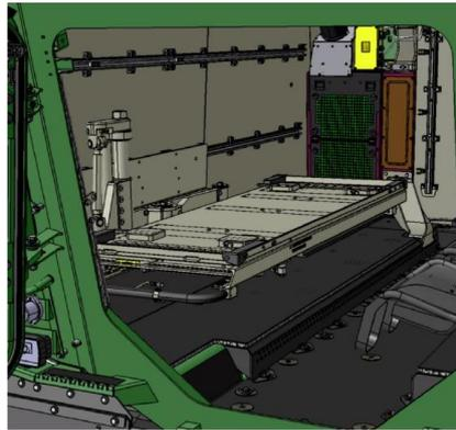
Figure 1-23 Stretcher installation in BvS10 rear car.
