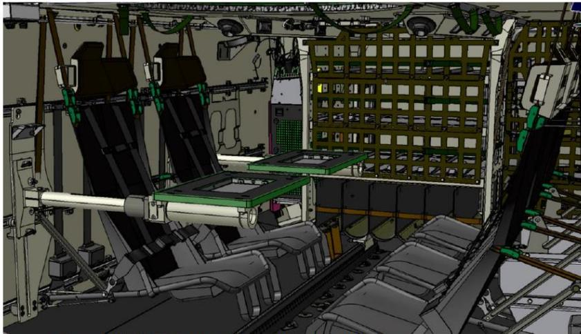
Figure 1-26 C2 kit (work tables) installed in the rear car.
